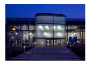
Pilkington Profilit™ is a U shaped profile glass. In standard configurations it is set within a perimeter aluminium frame in singular, double or triple glazed format. The modular nature of the system renders it a flexible design component perfect for inclusion within both exterior and interior projects.
